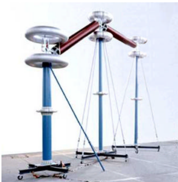
Fig. 1: HV capacitors used for voltage divider (right), HV filter and coupling capacitor
