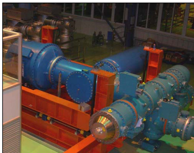
Fig. 3 (left): Metal-clad HVAC test system, type WP 400/800 G for routine testing of GIS spacers (courtesy of Hyundai)
