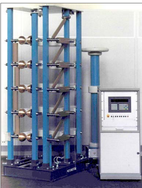
Fig. 1: Impulse voltage test generator IG 10/500 L
