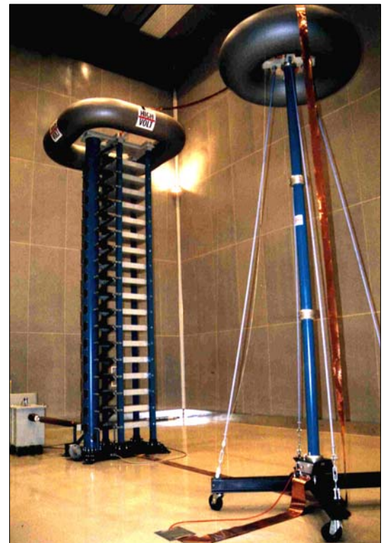
Fig. 1: Impulse voltage test generator IG 90/1800 M
