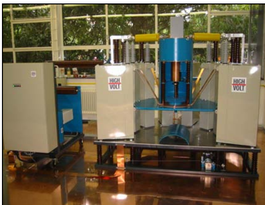
Fig. 2: Type IP 80/100 S; 80 kJ, charging voltage 100 kV; max. peak current 120 kA
