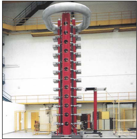
Fig. 7: Multi-stage Impulse voltage test generator (120 kJ/2400 kV) with modifications to produce currents up to 70 kA.
