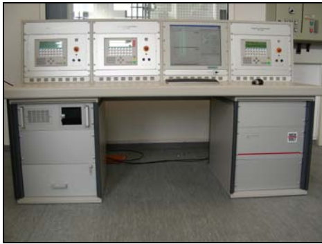
Fig. 5: Operator desk with control and measuring system for the impulse current generator IP 250/100 S shown in Fig. 3 & 4
