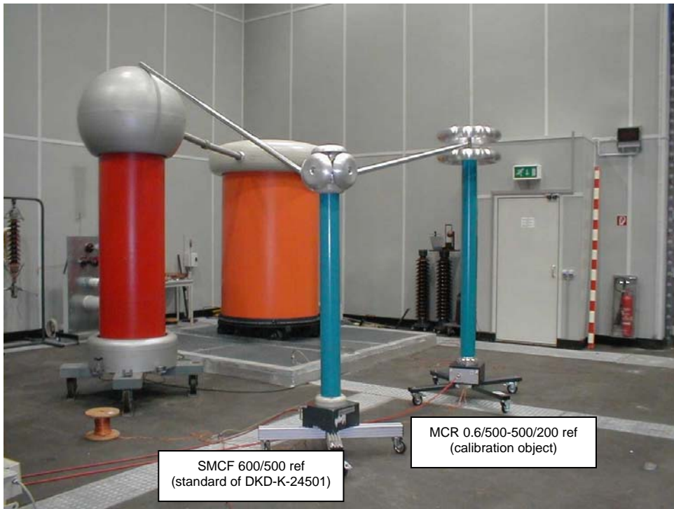
Fig. 2: Arrangement for comparison measurement for the calibration of RMS
