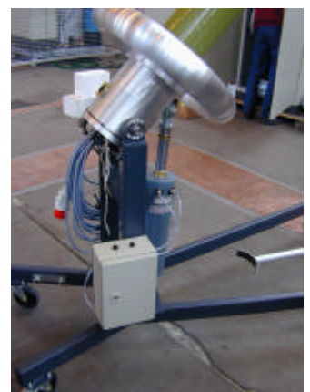
Fig. 3: CET 300/120 with motorized jacking system
