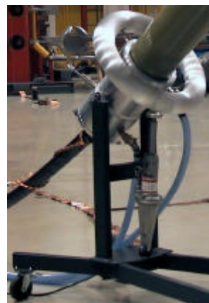
Fig. 2: CET 300/120 with manual jacking system
