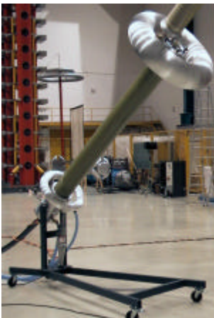
Fig. 1: View of a cable end termination for 300 kV, CET 300/120
