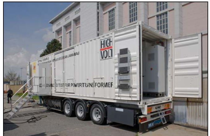
Fig. 4: 40 ft container for transformer test systems
