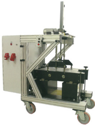
Figure 1: High-current transformer HCT 3000/15 B2
