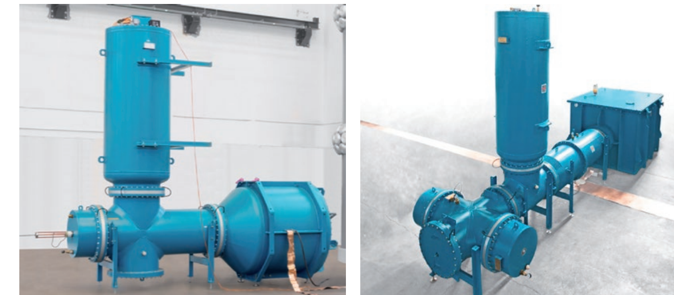
Fig. 1 AC test system WPG 500/750 G (gas-insulated transformer, left side) and WP 1000/500 G (oil-insulated transformer, right side)
