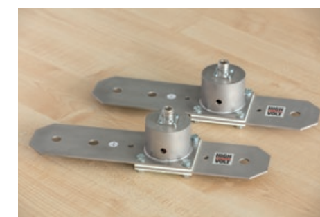
Fig. 11 Impulse current shunt usually used for impulse current measurement at dielectric tests on transformers
