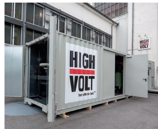
Fig. 7 Power Calibration System in a logistical standard 40-ft container
