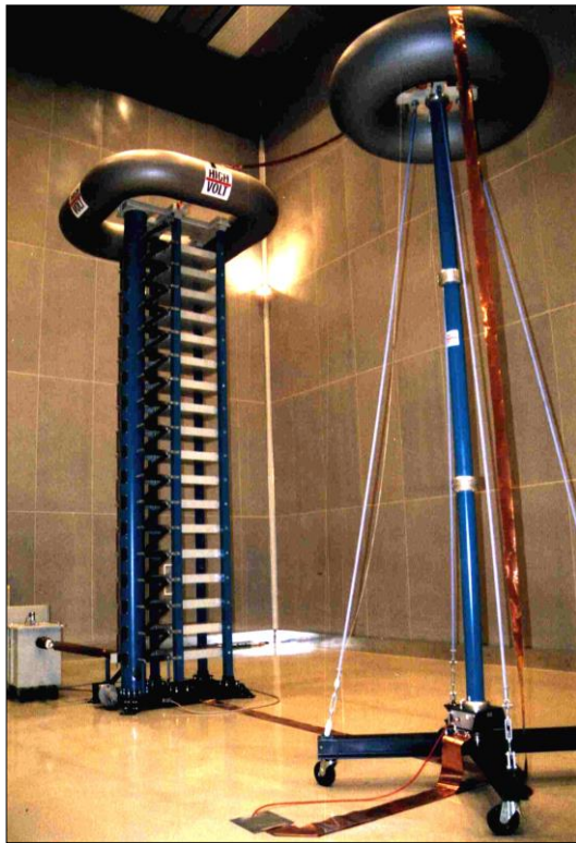
Figure 1: Impulse voltage test generator IG 90/1800 M
