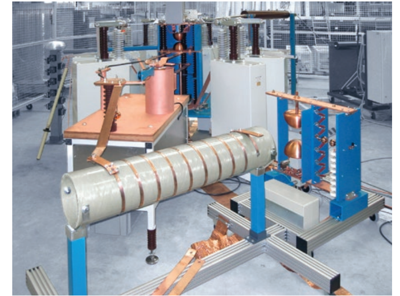
Fig. 4 Impulse Current Test System with impulse energy 128 kJ, charging voltage 80 kV and max. peak current 100 kA (10/350 \mu s) with additional crowbar circuit
