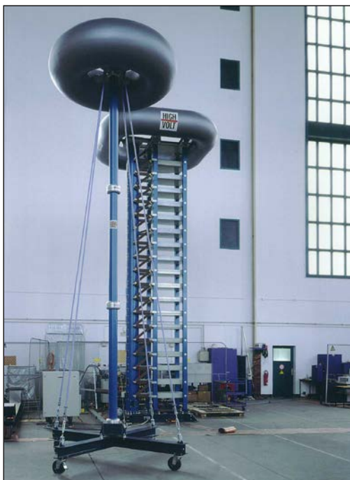
Figure 1: Impulse voltage test system, series M (SMC divider in the front)
