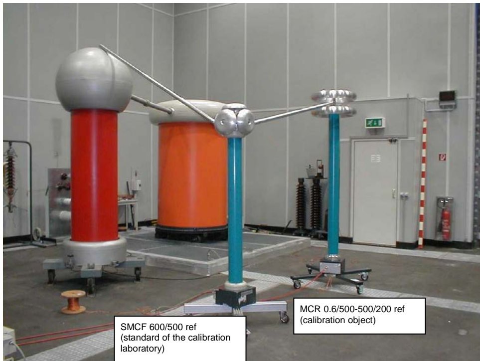
Figure 2: Arrangement for comparison measurement for the calibration of RMS
