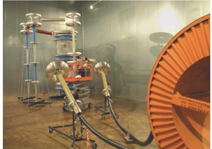
Fig. 2 Factory cable testing with HiRES Locator and AC resonant test system WRM
