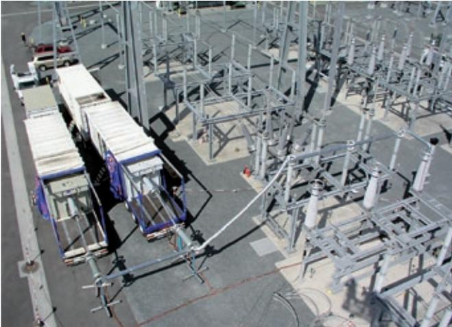
Fig. 3 On-site cable testing with HiRES Locator and AC resonant test system WRV 83/260 T
