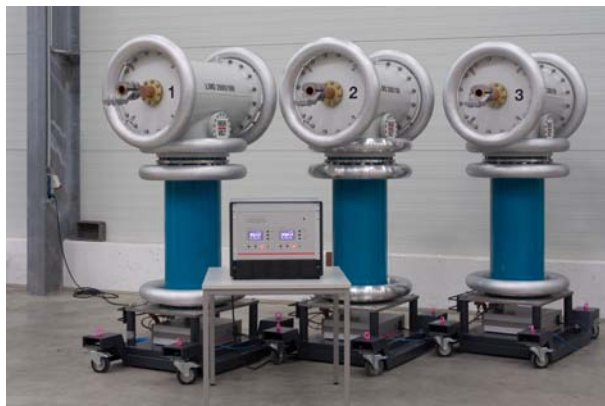
Fig. 2 Transformer Loss Measuring System LiMOS 2000/100-3 (with LiMOS MCSU; left: stand alone, right: integrated into operator desk)
