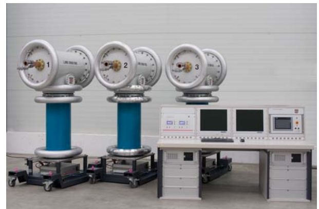
Fig. 2 Transformer Loss Measuring System LiMOS 2000/100-3 (with LiMOS MCSU; left: stand alone, right: integrated into operator desk)
