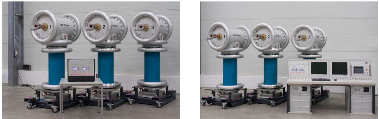
Fig. 2 Transformer Loss Measuring System LiMOS 2000/100-3 (with LiMOS MCSU; left: stand alone, right: integrated into operator desk)
