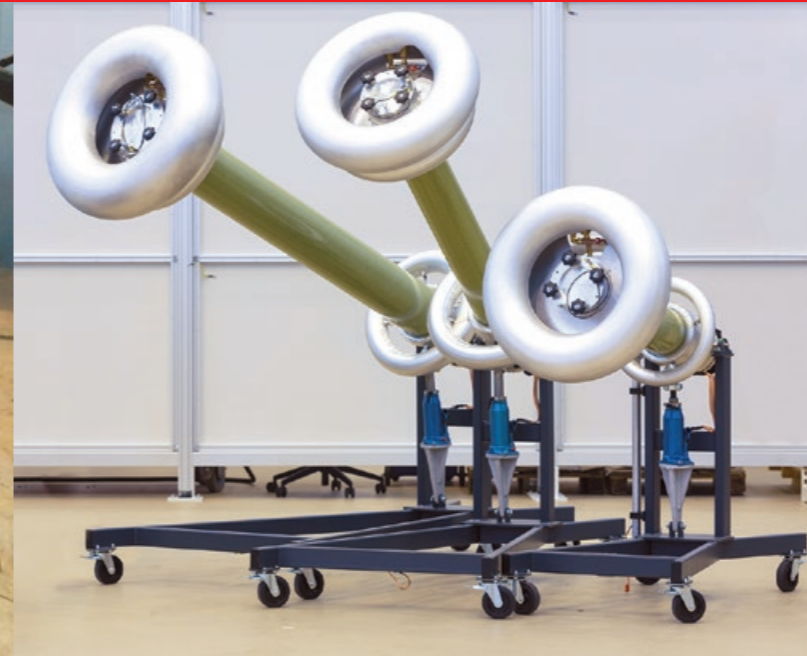
Fig. 3 Water-filled test terminations, type CET, several nominal voltages
