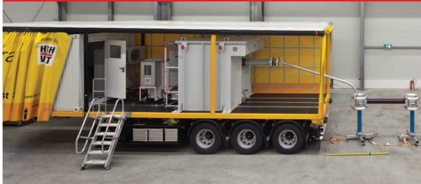
Fig. 1 AC resonant test system for on-site testing of extruded HV cables, type WRV 90/150 T
