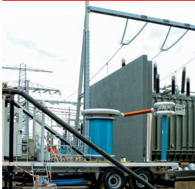
Fig. 1 Applied voltage test system for on-site testing of power transformers, type WRV 5/360 M
