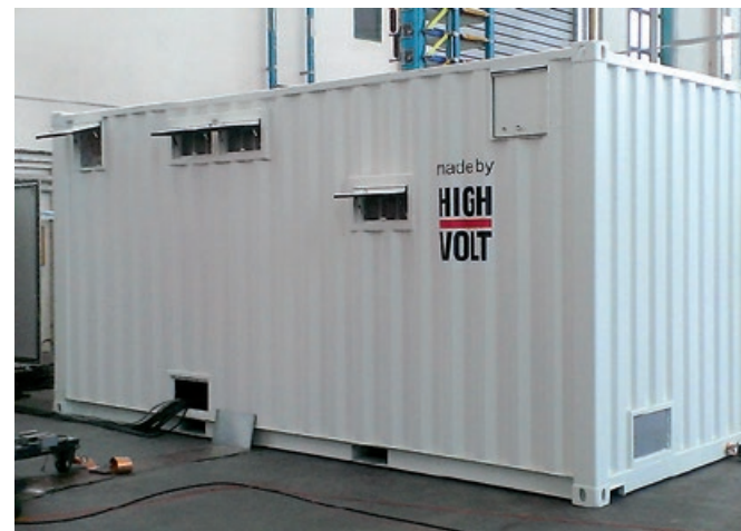
Fig. 2 Test system for small power transformers (left: test voltage source [SFC] in 20 ft container, right: loss measuring system LiMOS MS)
