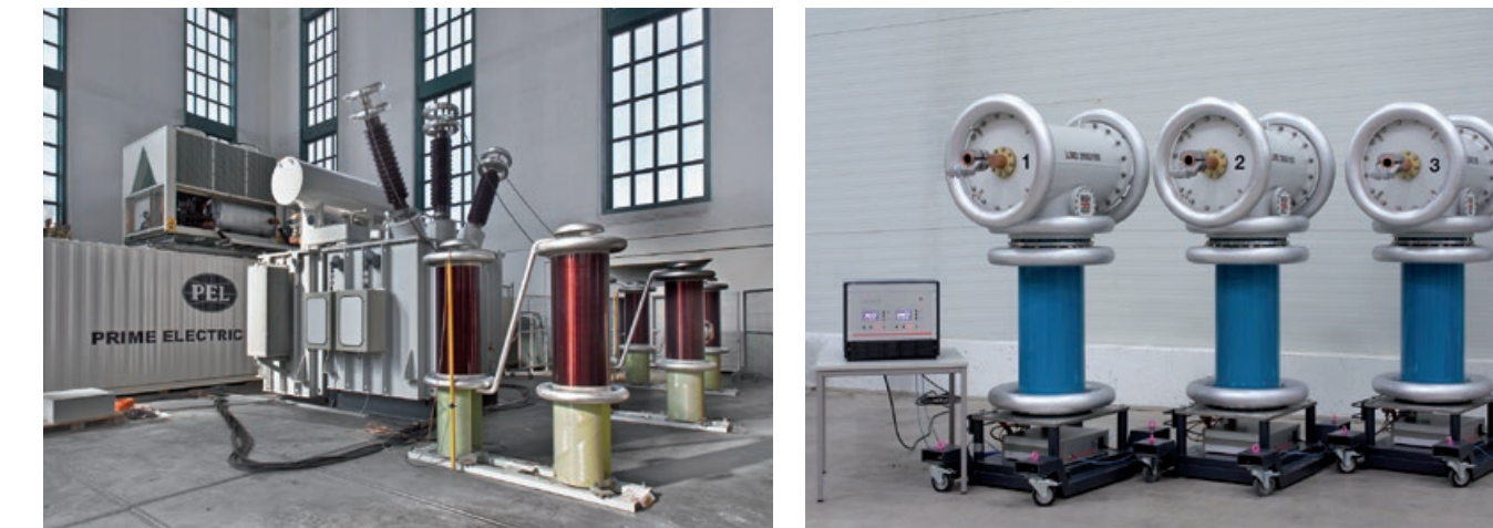
Fig. 4 Test system for large power transformers (left: 2 MW 4 MVA [SFC], tapped transformer and filters, right: loss measuring system LiMOS 2000/100-3)
