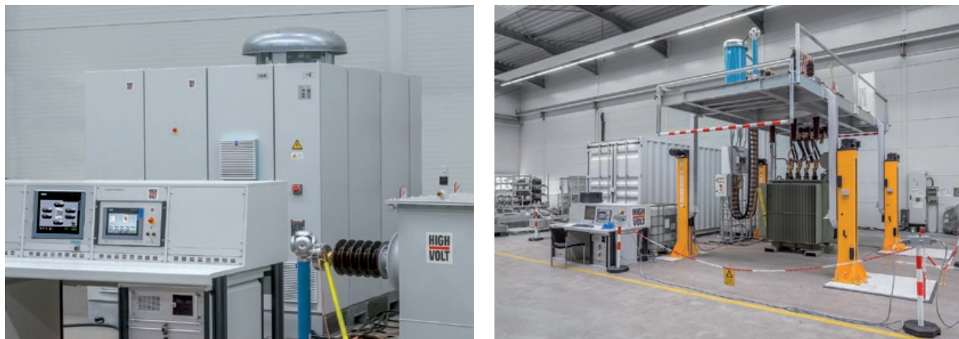
Fig. 1 Test system for type- and routine tests on distribution transformers (left: test voltage source and control system, right: automatic switching system)
