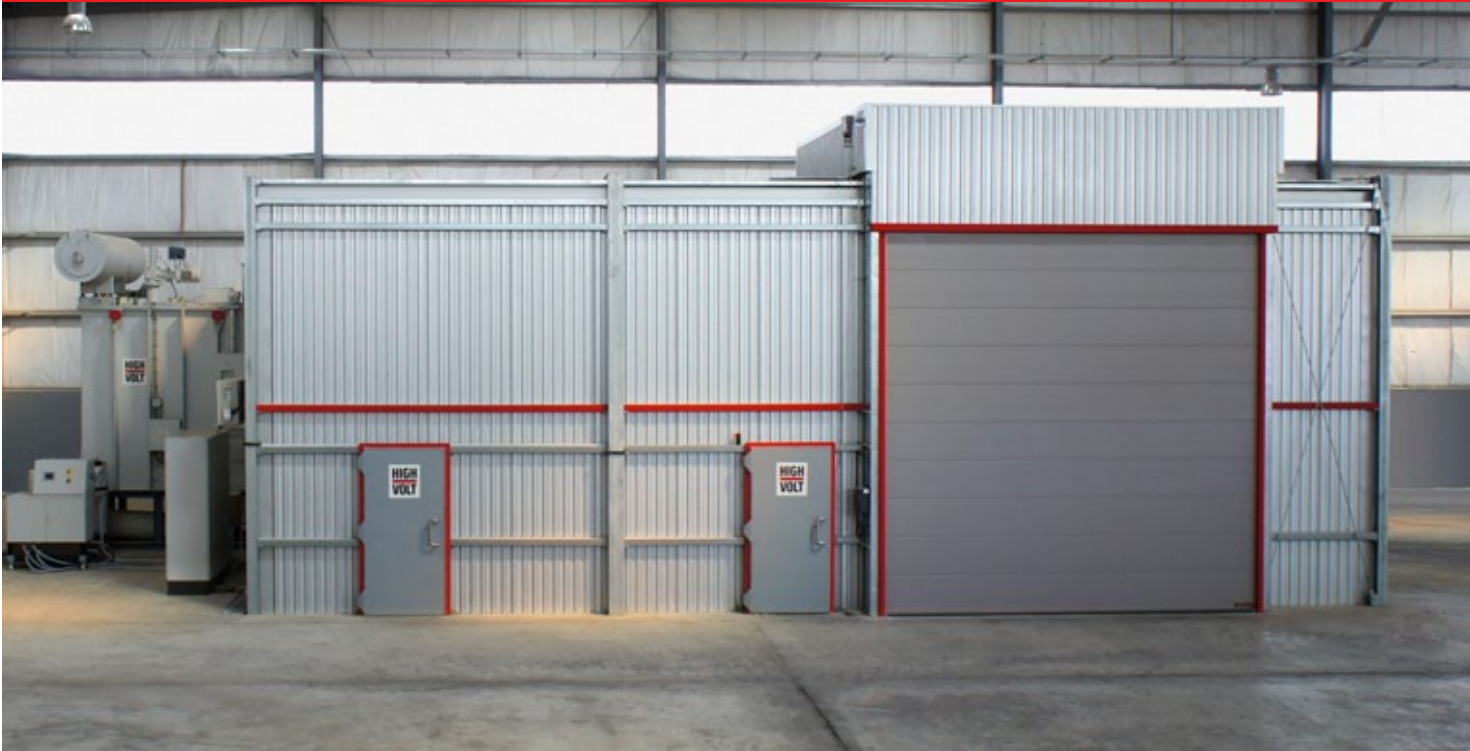
Fig. 1 Shielded room SSC 15/9/5.6 with integrated AC resonant test system WRU 10000/350-200-100 for routine testing of high-voltage cables
