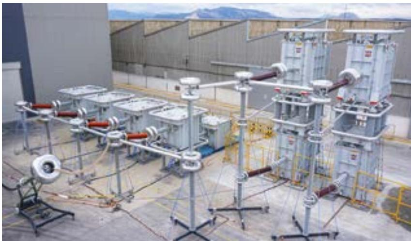
Fig. 1: Four new reactors DE 120000/225-122 (right) combined with 8 conventional reactors, resulting in an installed total test power of 700 MVA – the most powerful testing system in the world to date.
